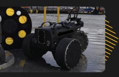
Inspect Entire JPU GRAKO's remote semi-autonomous abilities can inspect an entire JPU, capturing high-resolution images and storing them in a single file for convenient post-inspection review. COREMATIC's solution provided the mining company with a fast and accessible way to address their inspection needs.
